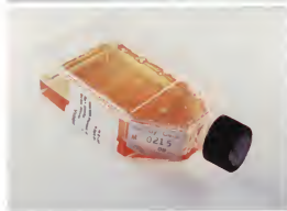
16-6, 7 Tissue culture flasks. Plastic or glass flasks of different sizes can be utilized to grow cell monolayers or cells in suspension. Once the flasks are seeded, they are placed inside incubators.
